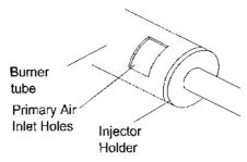
Figure 21 - Injector Holder On Outlet Burner Tube
